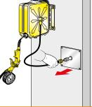
To prevent removal or theft of the hose reel it can be locked with a bolt or padlock
